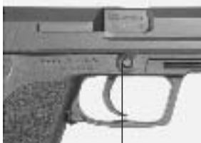
Lage Verschlussfanghebelachse Position of the axle of the slide release
