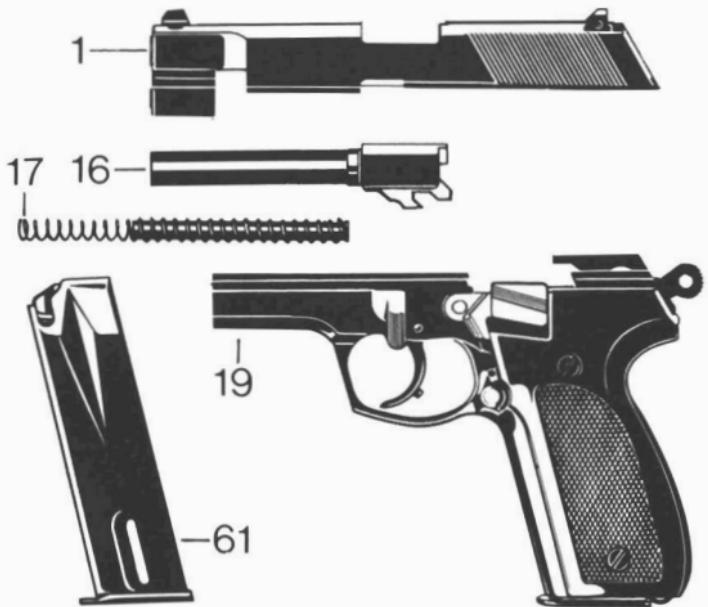
Press the recoil spring guide forward and lift it out with the recoil spring. Now, the barrel can also be taken out.
